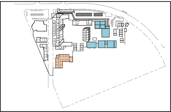
Phase 2 Construct locker room building. Convert old locker room into additional PE facilities. Install AC into both gymnasiums. Replace HVAC in Building S. Demolish Building H and remove two portables.
