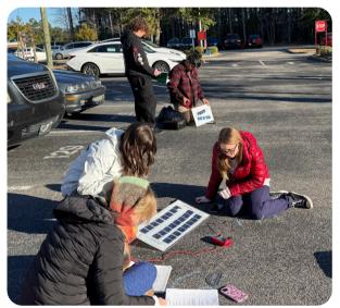
Environmental engineering juniors finished building their solar panels this week and did their final tests outside in the sunshine. Students used a compass, protractor and multimeter to find the solar elevation and azimuth angles that produced the most voltage. The graphed their results to analyze the role angles play in solar panel efficiency.
