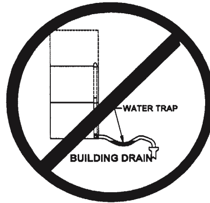
IMPROPER DRAIN LINE CONNECTION
