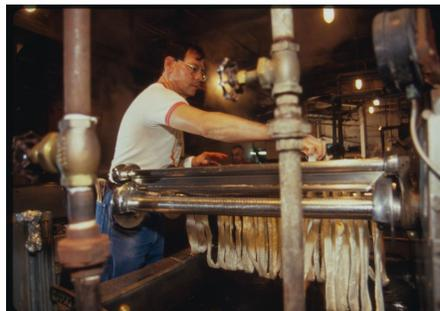
Machine operator at work at a silk skein dyeing tank. Working in Paterson Project, 1994.
