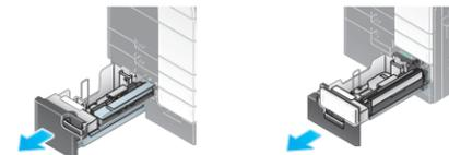
2. Lift up the paper take-up roller, and then load the paper into the tray.
