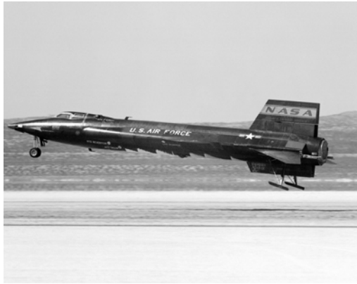
The X-15 hypersonic research aircraft was instrumental in the development of the human spaceflight programs that followed. Courtesy of NASA
