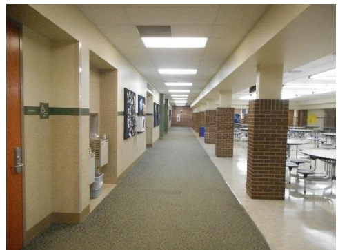
Typical carpeted corridor and VCT cafeteria
