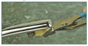
One or more parts are contained within the aerator. Note the order and orientation of the parts as you remove them;
