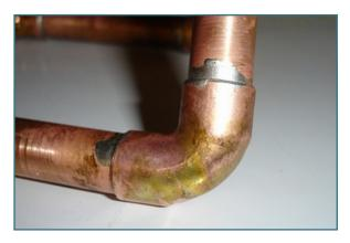
Copper pipes joined by lead solder.
