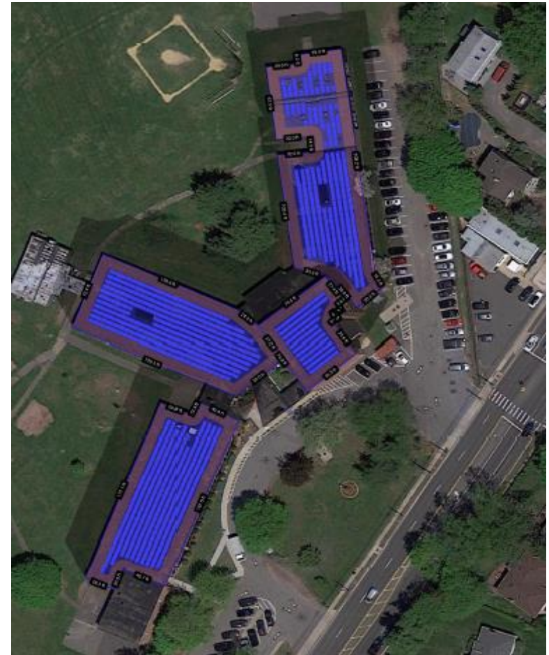
Baylis Elementary School – 282.4 kW Design
