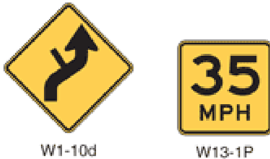
Image 5 – DRIVEWAY ON CURVE and ADVISORY SPEED signage
