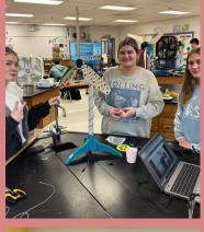
Clean energy juniors researched, designed, created, and tested some fantastic wind turbine blades! They first maximized voltage and efficiency for electrical power. Next, they put their turbines to work pumping water, lifting weights, and lighting some LEDs.
