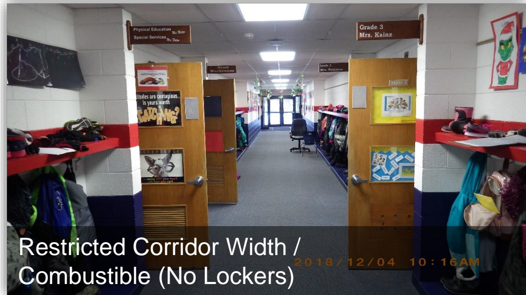
No Fire Suppression System Wood Framed Walls Not Allowed
