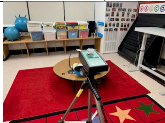
View of Room 32 Location of Mold Air Sample 38526955.
