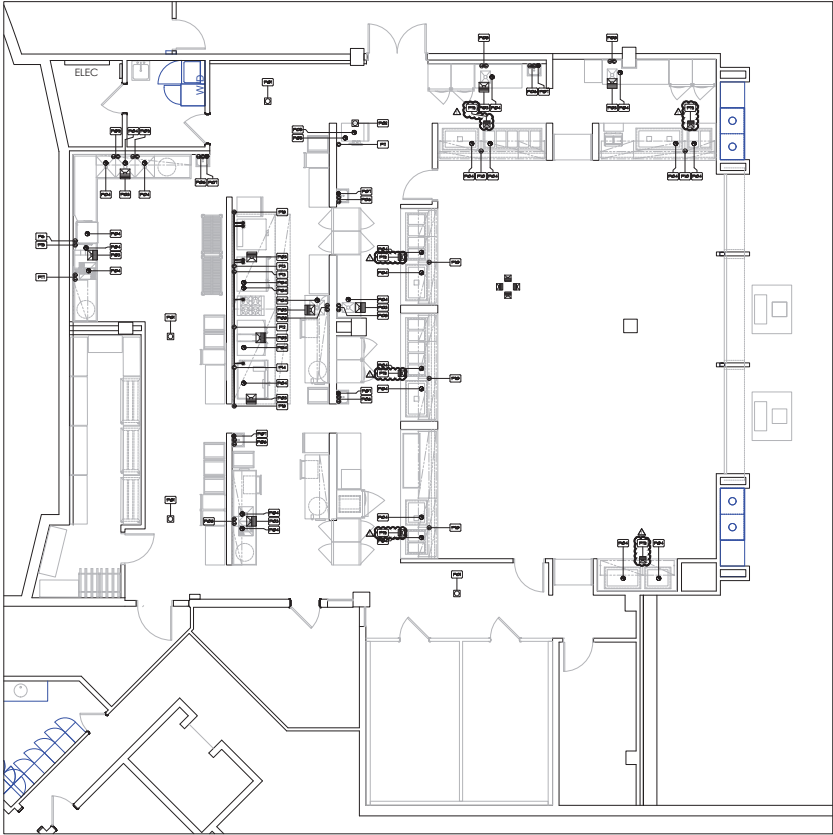
1 FOODSERVICE EQUIPMENT PLUMBING CONNECTIONS PLAN 1/4" = 1'-0"
