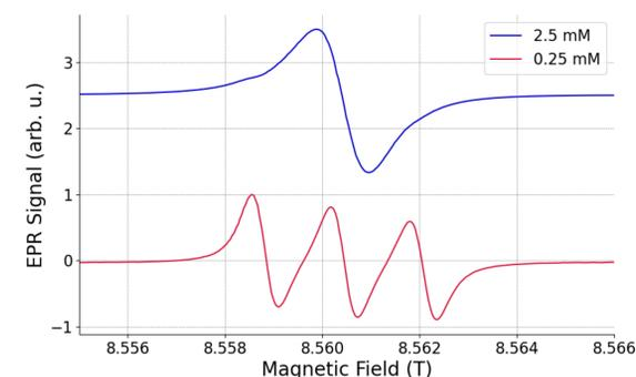
FIG. 11. EPR signal of 2.5 mM and 0.25 mM of TEMPO dissolved in toluene
