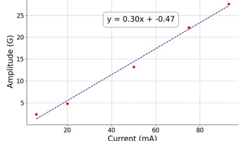
FIG. 9. The modulation coil amplitude as a function of the current. The dashed line represents the linear fit
