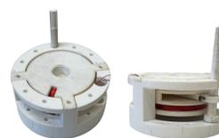
FIG. 12. Two-cell sample holder printed from polylactic acid using the Original Prusa i3 MK3S+ 3D printer
