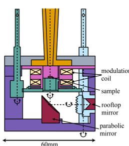
FIG. 5. Diagram of the quasi-optical sample holder (adapted from [7])
