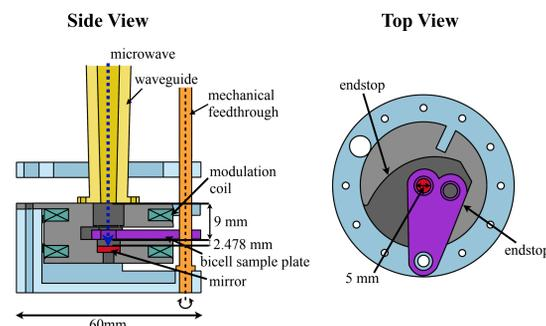
FIG. 6. Proposed design for the 3D printed two-cell sample holder and modulation coil
