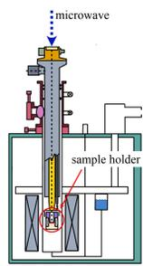
FIG. 1. Diagram of EPR probe inside the superconducting cryogen-free magnet (adapted from [4])
