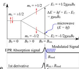
FIG. 3. Diagram showing the interaction between an electron spin ( $S = 1/2$ ) with an external magnetic field,  $B_0$ , and the frequency ( $f$ ) of an oscillating electromagnetic irradiation. When the microwave radiation matches the gap at the absorption signal, the lower energy levels flip to a higher energy level [4]
