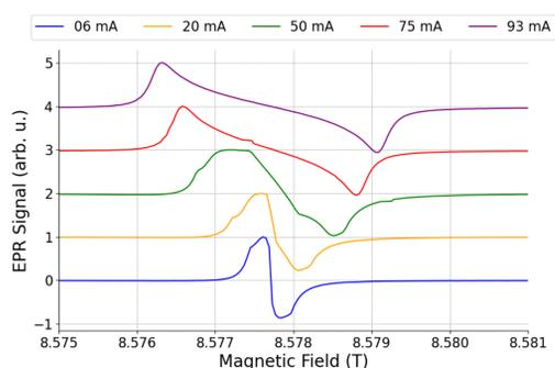
FIG. 8. The difference in linewidths of the LiPc crystal at five currents: 6, 20, 50, 75, and 93 mA
