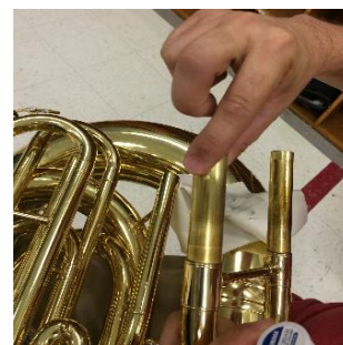
Applying slide grease w/ finger
