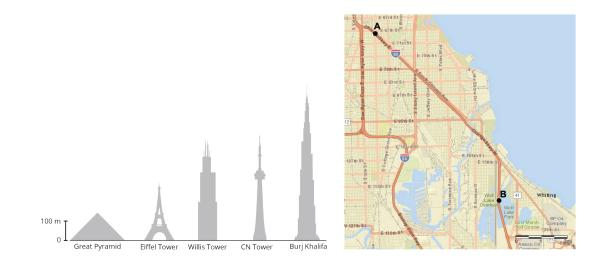
The **scale** tells us what some length on the scale drawing represents in actual length. For example, a scale of "1 inch to 5 miles" means that 1 inch on the drawing represents 5 actual miles. If the drawing shows a road that is 2 inches long, we know the road is actually  $2 \cdot 5$ , or 10 miles long.
