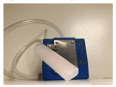
The 4-polycyclohexene (4-PCH) samples were collected in SKC's Anasorb CSC sorbent tubes through Gilian GilAir3 Air Sampling Pumps (photograph below). Pumps were placed within the breathing zone (4-6ft from ground level). Run times were 8 hours or time-weighted 4-hour runs. 4-PCH analytical results can be found in Appendix E.
