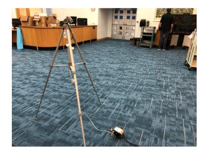
Radon gas samples were collected by securing Air Chek Radon Test Kits (photograph below). Samples were collected within the breathing zone (4-6ft from ground level) at each sample location. In accordance with Air Chek's Radon Test Kit Instructions, kits were secured to walls inside the building and away from open windows, doors to the outside, or interior air ventilation systems. The sampling time was 72 hours. Radon analytical results can be found in Appendix B.
