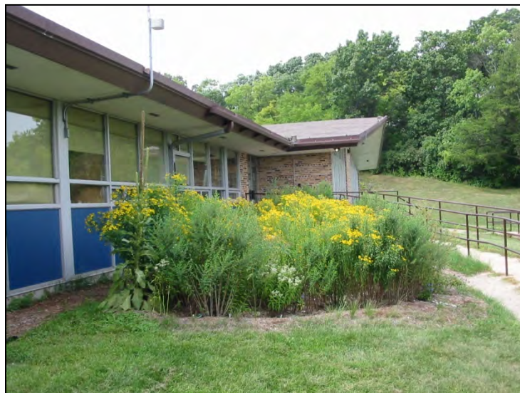
Example of a rain garden utilizing natural vegetation and eliminating the cost of lawn maintenance.
