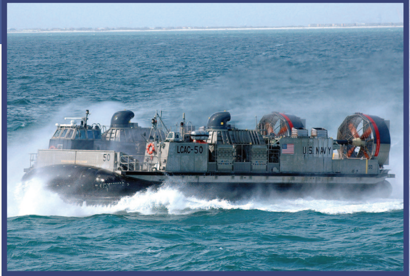
The LCAC travels across the water on a cushion of air.
