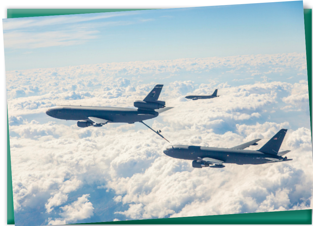
A KC-46A ( right ) undergoes testing of its own refueling system. Here it receives fuel from a KC-10 extender, with a KC-135 off in the distance.
