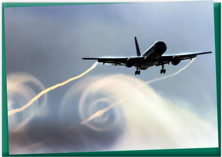
Wingtip vortices on display during takeoff.
