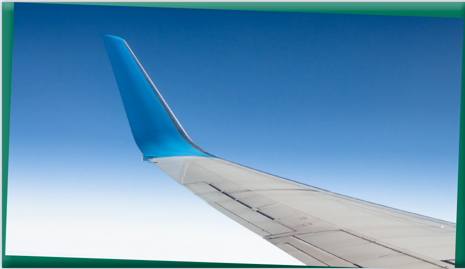
The winglet is used to reduce induced drag and wingtip vortices.
