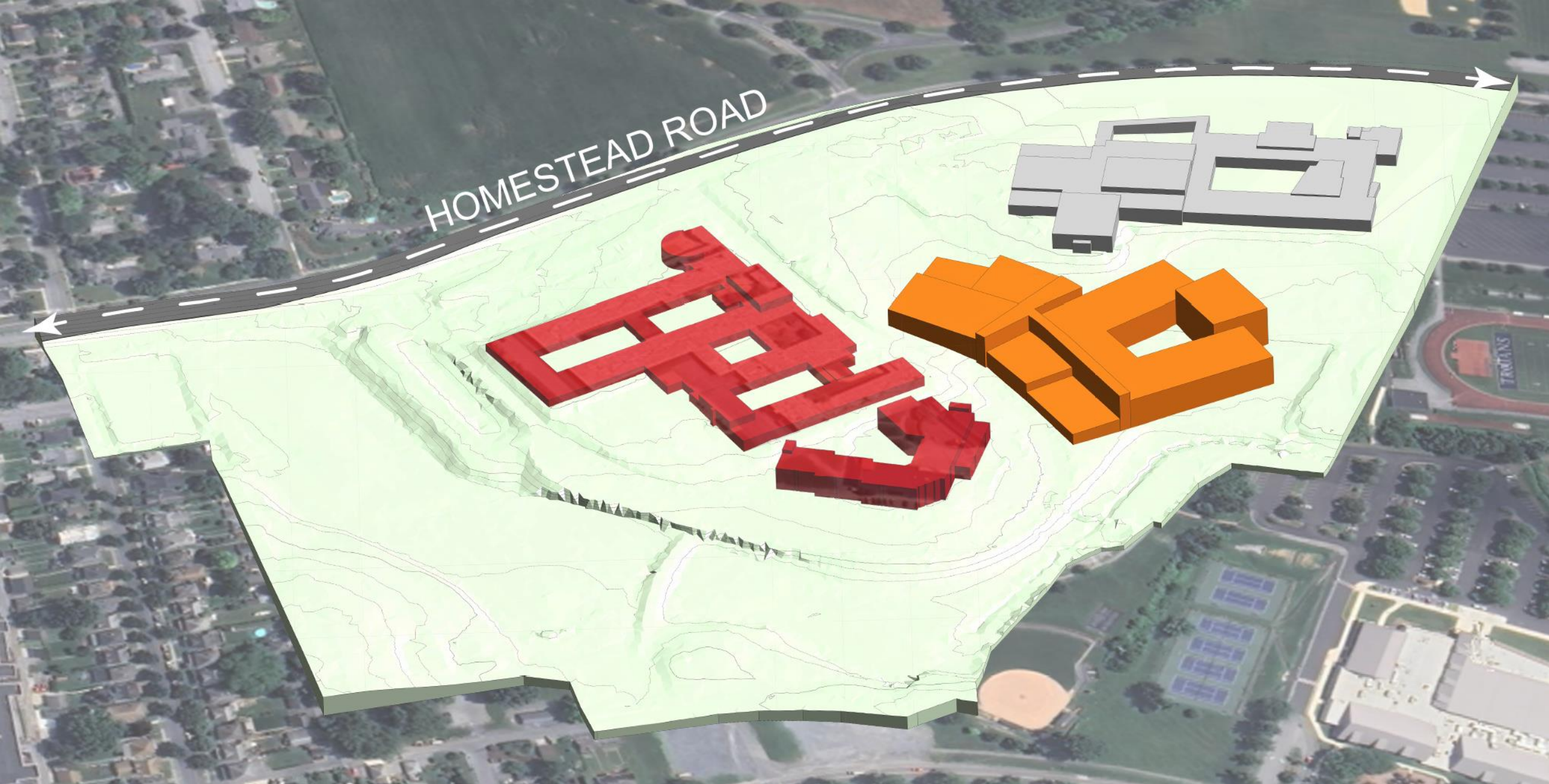
Phase 2: Demolition of ES and ECC
