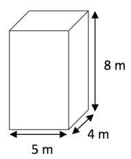
Volume =  $5 \text{ m} \times 4 \text{ m} \times 8 \text{ m} = 160 \text{ m}^3$
