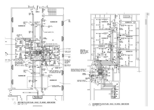
In 2017, the unit ventilator was replaced with new dual temperature unit ventilators. A decoupled rooftop ventilation unit was added to serve the entire wing. A small variable refrigerant flow system was provided to serve offices on the second floor. The mutlizone air handling unit was also replaced as part of this project.
