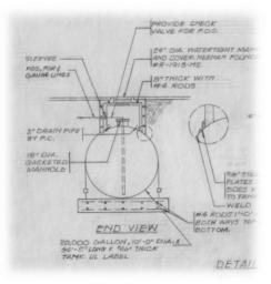
Detail of Original Fuel Oil Storage Tank (Replaced in 1993/1994)
