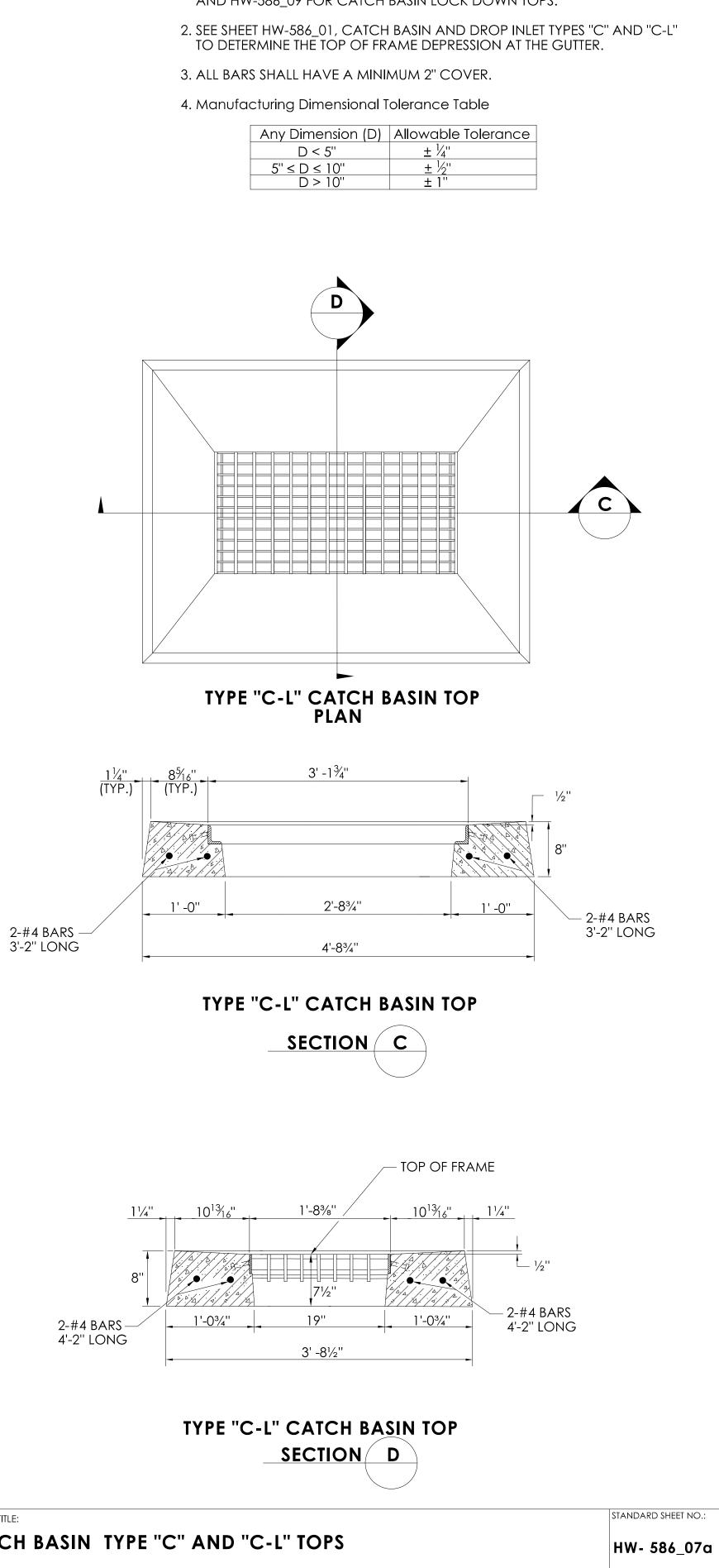
1. SEE SHEET HW-586\_08, FOR CATCH BASIN FRAMES AND GRATES AND HW-586\_09 FOR CATCH BASIN LOCK DOWN TOPS.
