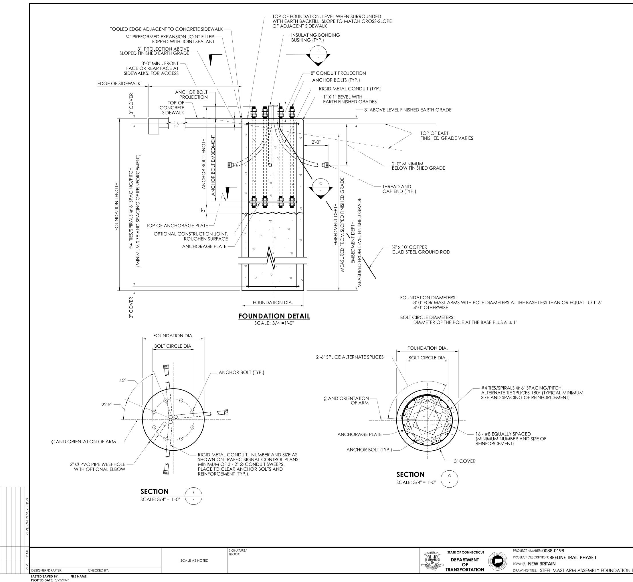
THE DRILLED SHAFT FOUNDATION FOR THE MAST ARM ASSEMBLY SHALL BE DESIGNED, FABRICATED, AND CONSTRUCTED BY THE CONTRACTOR IN ACCORDANCE WITH THE SPECIAL PROVISION "TRAFFIC CONTROL FOUNDATION - MAST ARM".
