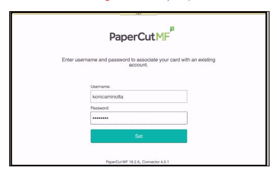
Press Ok. Then Press the Machine Reset Button. You Now Can Use Your Card to Access the Konica Minolta Device.
