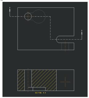
8. Go to Sketch Tab > Select Circle Tool > From Snapping Pop Menu Select Arrow Reference > Select the Center Line and one of the hidden lines from the top view that represent the Circle > Middle Mouse Button to deactivate the reference tool > Place Cursor at center of centerline cross in the front view place circle > With Circle selected Reference circle to View.
