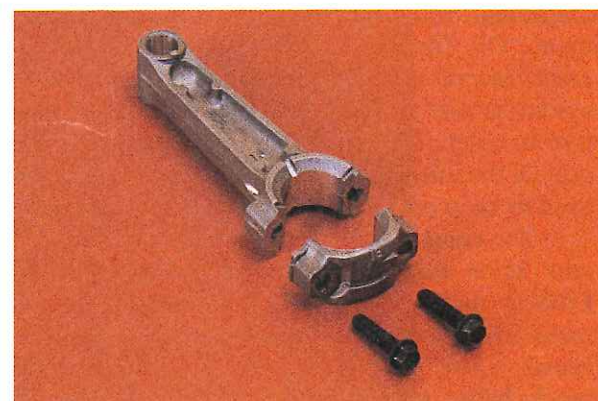
Figure 4-18. Shown are the relative positions of connecting rod parts.
