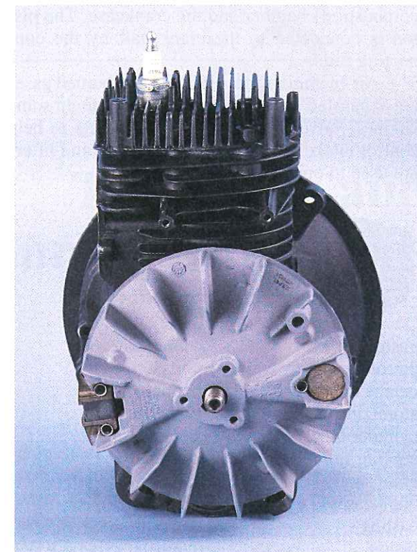
Figure 4-31. The flywheel is fastened to the crankshaft. When rotating, its weight smoothes engine operation.
