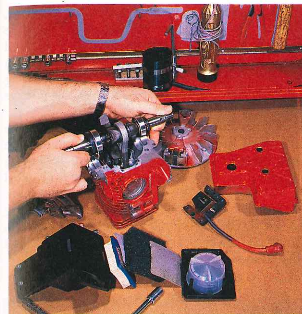
Figure 4-13. The crankshaft must be clean and carefully installed in the crankcase. The tapered end fits into the flywheel, which is secured with a key, lock washer, and nut. (Tecumseh)
