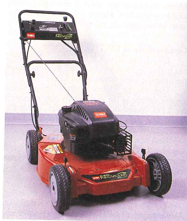
Figure 7-6. On this lawn mower the plastic fuel tank is contoured to fit snugly around engine.
