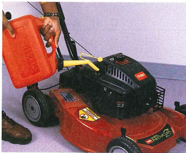
Figure 7-2. Refueling a four-cycle engine requires use of an approved fuel can and a fresh fill of regular gasoline.
