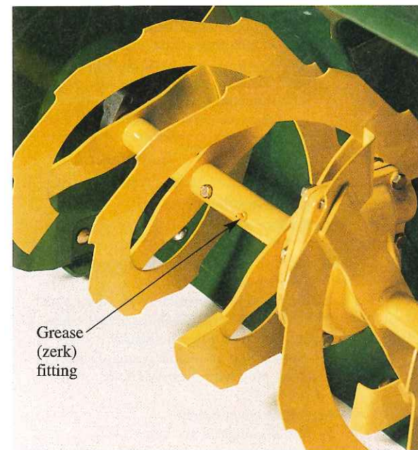
Figure 20-38. Shown is the grease (zerk) fitting located on the auger shaft. (Deere & Co.)
