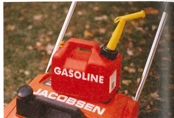
Figure 20-2. Gasoline should be stored in an approved and clearly marked container. Never store gasoline, or other flammable liquids in glass containers. Refuel outdoors away from any flames. (Jacobsen Manufacturing Co.)
