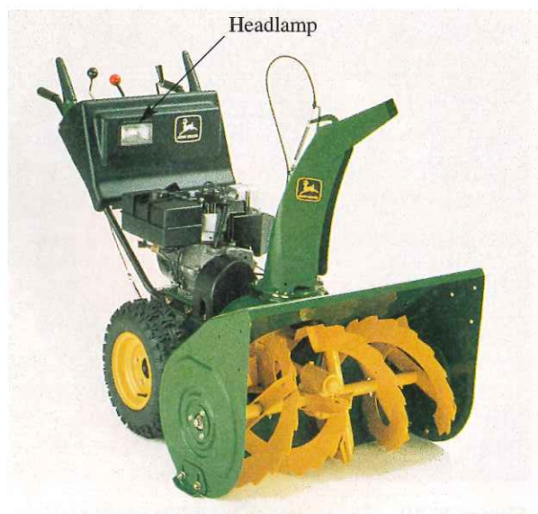
Figure 20-12. This model has a sealed beam headlamp for night work. Unless the electrical system is voltage regulated, the light will brighten and dim as engine speed varies. (Deere & Co.)
