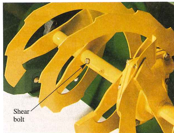
Figure 20-36. Each auger blade has a shear bolt or pin that protects the auger gear box from damage resulting from an obstruction in the auger housing. (Deere & Co.)
