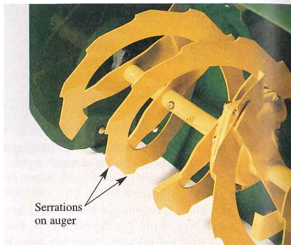
Figure 20-14. An auger with serrated edges can break up ice and snow into finer particles before it enters the second stage blower. (Deere & Co.)
