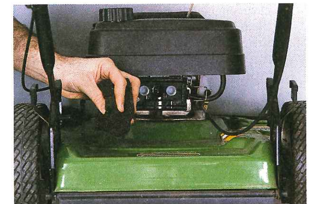
Figure 8-48. This polyurethane foam filter can be removed, cleaned, and reoiled.
