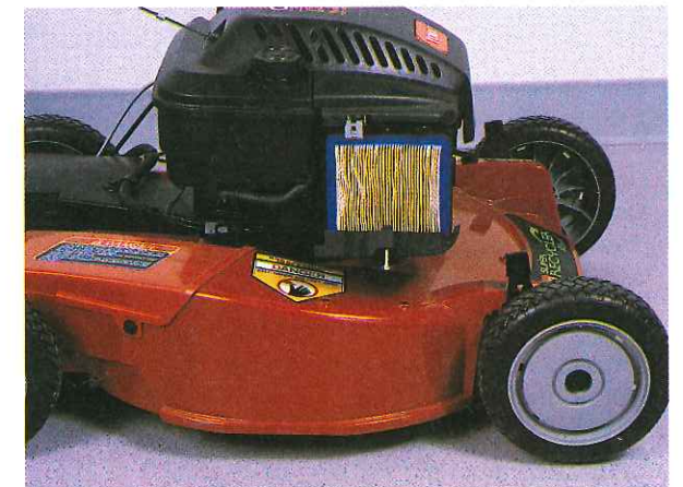
Figure 8-53. When installing the pleated paper air cleaner cartridge, place the paper element toward the external cover side of the receptacle.
