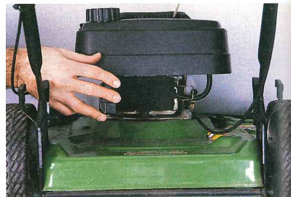
Figure 8-46. An oil-wetted air cleaner. Polyurethane foam is dampened with oil and contained in a vented case attached to carburetor.
