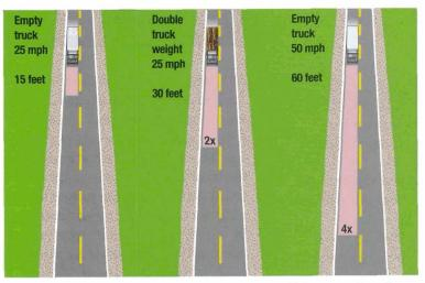
A vehicle's energy of motion increases dramatically with increases in weight and speed.
