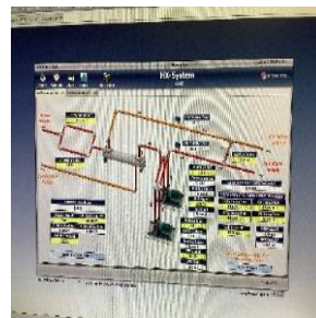
Steam to hot water heat exchange system dashboard
