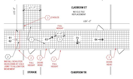
B. The 4 ft. patch (Keynote #3) at Cross Corridor 1/A-102 revise to "INSTALL BACK-TO-BACK J-MOLD TRIM AND REPAIR PLASTER AND CAULK JOINT. PAINT WALL CORNER TO CORNER. In the same area, on South wall, patch and repair plaster above doors at 4 locations (approx. 4 sf each). Paint from corner at Cross Corridor to logical stopping point above door at Classroom 157.
