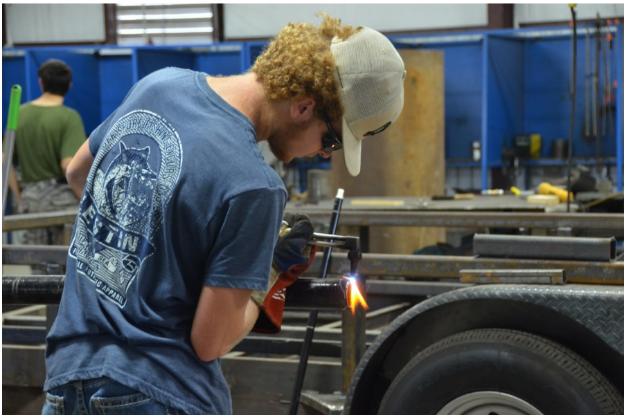
Colton Jamison (11) uses a cutting torch to saddle pipe for the duck blind he and Andrew Jacobus (11) are building for the Yamboree Ag Mech show. PHOTO: Bre Reynolds
