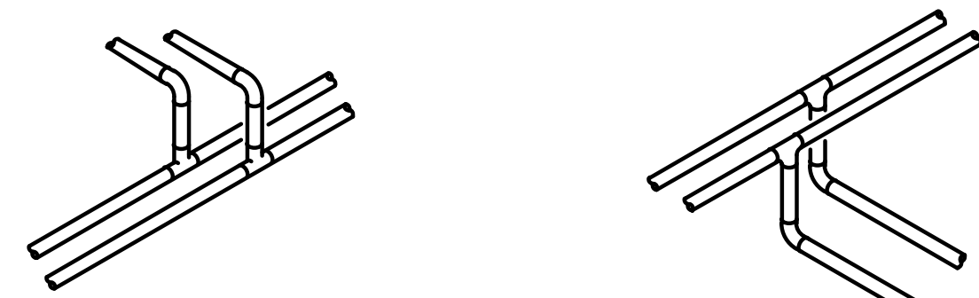
BRANCH CONNECTION OFF TOP APPLIES TO THE FOLLOWING SYSTEMS: DOMESTIC WATER STEAM & CONDENSATE LABORATORY GASES LABORATORY VACUUM COMPRESSED AIR NATURAL GAS BRANCH CONNECTION OFF BOTTOM APPLIES TO THE FOLLOWING SYSTEMS: HOT WATER HEATING CHILLED WATER CONDENSER WATER ENERGY RECOVERY PROCESS COOLING WATER NOTE: BOTTOM AS INDICATED OR SIDE CONNECTION IS ACCEPTABLE. CONNECTION ABOVE CENTERLINE OF MAINS IS NOT ACCEPTABLE.
