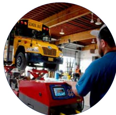
New hydraulic lifts in mechanics' bays allow safe access underneath buses
