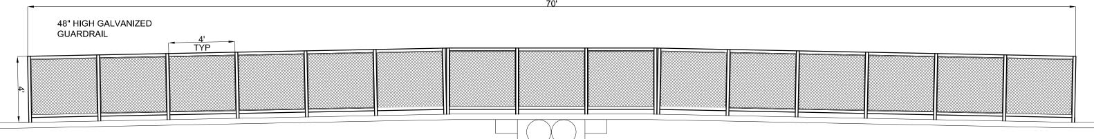
\* Factory welded rail constructed of 2" x 2" x 14 ga. square tubing and 1/2" square vertical rods welded on 4" centers.
