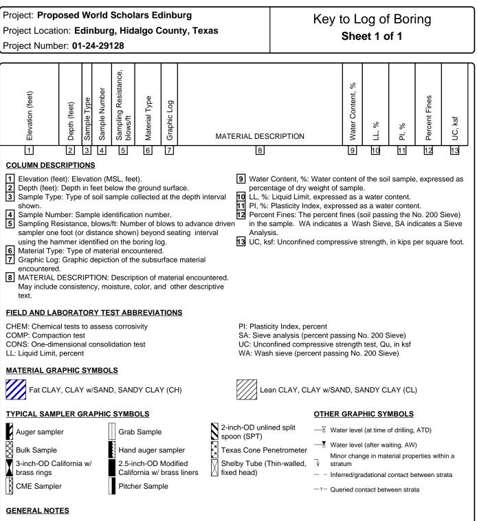
1: Soil classifications are based on the Unified Soil Classification System. Descriptions and stratum lines are interpretive, and actual lithologic changes may be gradual. Field descriptions may have been modified to reflect results of lab tests.
