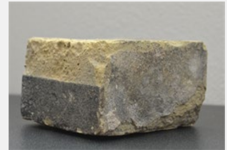
The effects of sandblasting – the top part of this brick has been sandblasted, removing its outer layer and causing further damage to the lower part of the brick. Photo by Ginny Way, courtesy of Wisconsin Historical Society.
