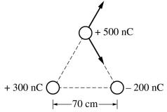
As shown above, the vertical components of the forces subtract and the horizontal components add.
