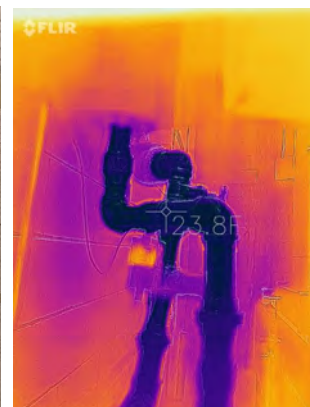
Thermograph of uninsulated hydronic piping
