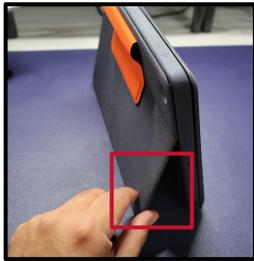
3. Lower the front **keyboard flap** to have access to the keyboard and trackpad.
