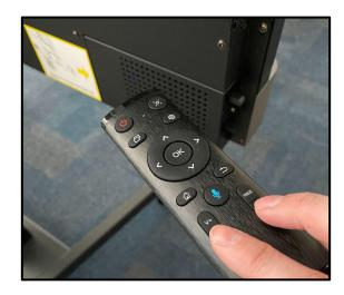
3. Press the V- and BLANK buttons at the same time, and the indicator light will start flashing.
