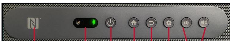
1. **NFC Sensor:** Tap NFC card here to login or tap the end of the panel pen to activate EZWrite.
