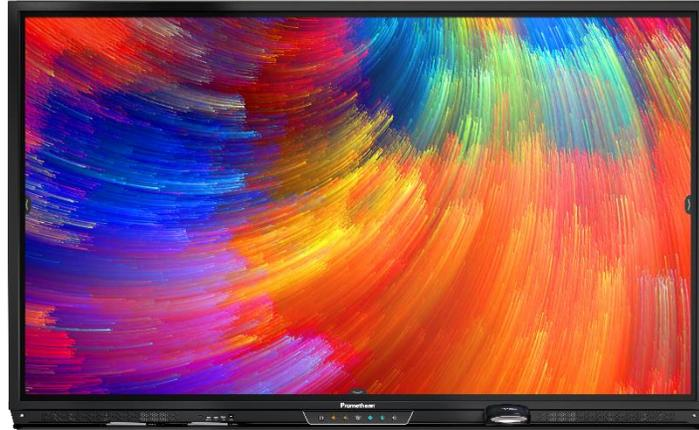
The front of your ActivPanel Titanium features a center console, positioned for comfort and easy accessibility at a 30-degree angle. Use the Center Console to adjust the volume, access the Unified Menu, manage touch on and off and freeze, as well as switching sources.
