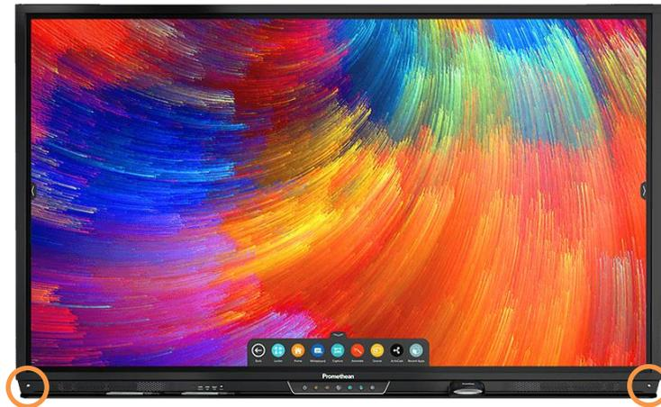
As you enter the room and near the ActivPanel, the dual proximity sensors automatically begin the boot up process.
