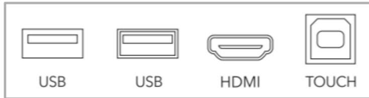
You will find additional ports on the back of your ActivPanel. When facing the panel, they are on the left side. Be sure to connect HDMI and USB cables into their corresponding ports. For example, use **HDMI 2** in tandem with **TOUCH 2**.
