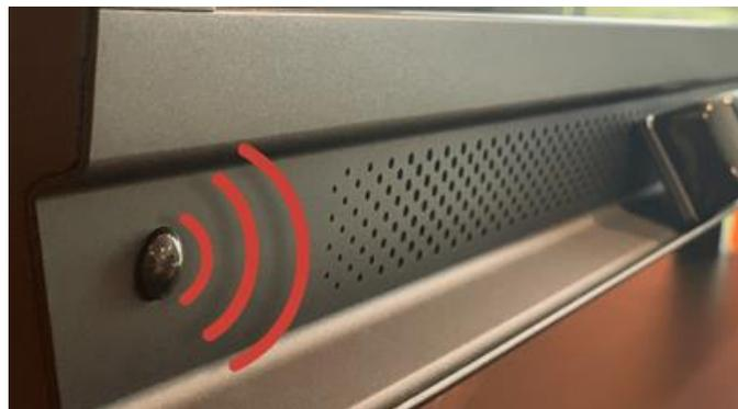
To instantly power on the panel, simply touch the **power button** on the center console.
