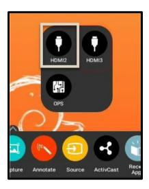
Note: The Chromebox is usually plugged into HDMI 2 or HDMI 3. If another Source does not "pop-up", you may need to press the power button on the Chromebox. It is a small rectangle that will display a white light when the Chromebox is powered on.
