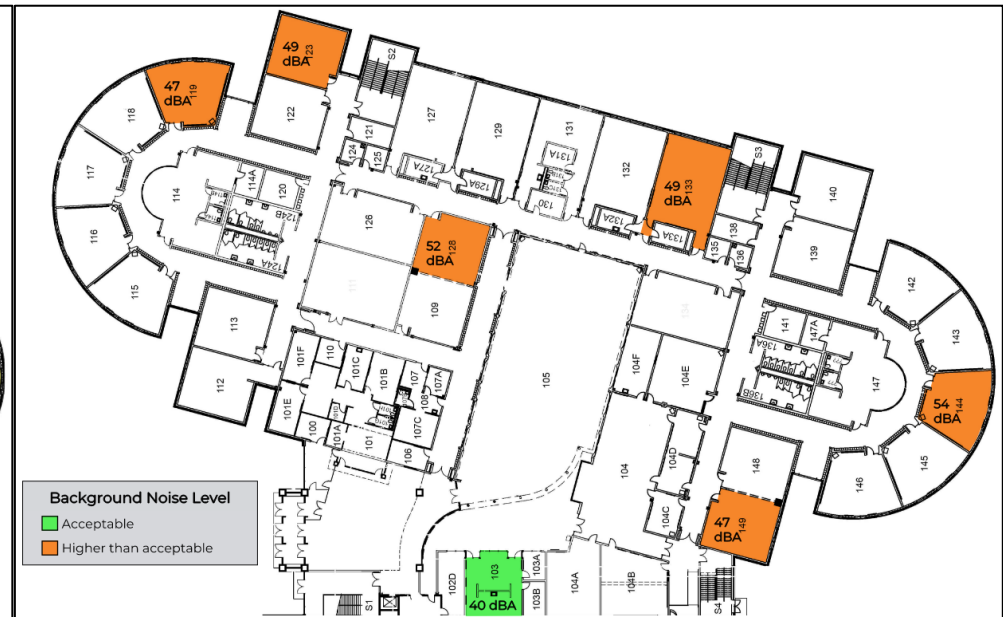
Figure 1: Upper St. Clair High School First Floor Sound Level Readings (dBA)
