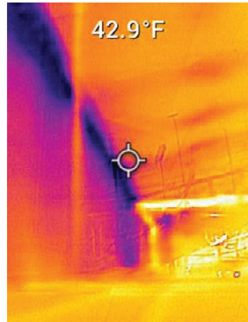
Fig. 6&7 – Interior ceiling plenum at exterior wall. The CMU to gyp is sealed but IR shows significant thermal leakage where the concrete meets the roof.
