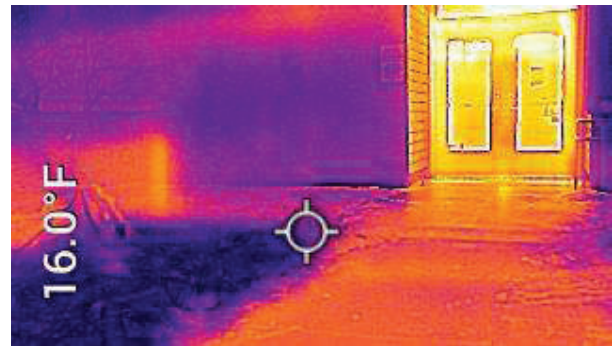
Fig. 2&3 – East entry upper level. IR shows some thermal leakage where the concrete meets exterior wall.
