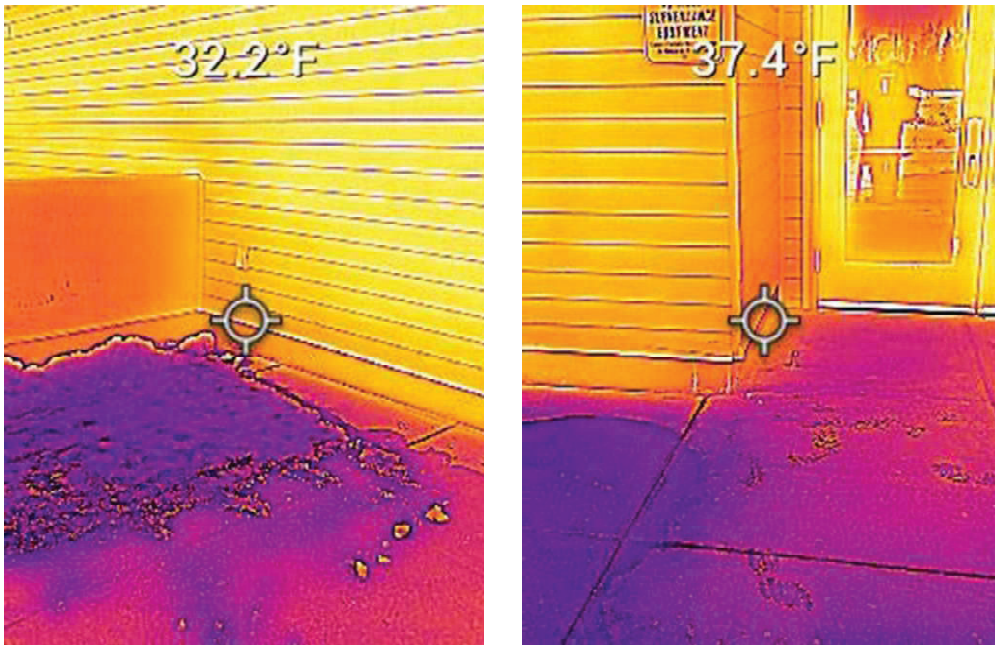
Fig.15&162 Upper SE Classroom wing Entry – thermal transfer at wall base.
