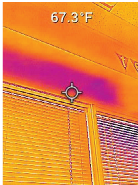
Fig.13&14 Upper SE Classroom Window – area of leakage has noticeable darker areas. This indicates damaged insulation.
