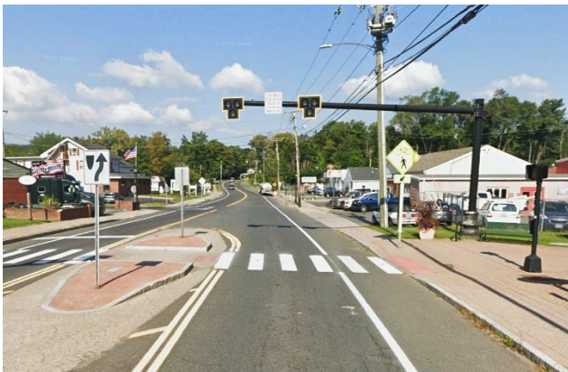
Figure 8-13: Crosswalk with median refuge island and a Pedestrian Hybrid Beacon. Cheshire, CT. Image Source: Google Street View
